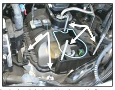
**4.** Set the throttle body and brackets aside. Remove the factory throttle body studs. Install two 6mm x 114mm studs (#2) in the front mounting holes, and one 6mm x 70mm stud (#3) in the rear. Using 4mm and 10mm sockets, remove the factory throttle cable bracket studs.
