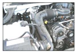
**8.** Re-install the intake tube, and tighten the hose clamps. Re-connect the breather hose elbow to the intake hat. **Re-connect the negative battery cable!**
